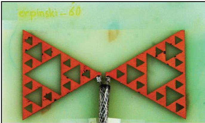
Fig. 17. The fabricated S3-60° antenna.
