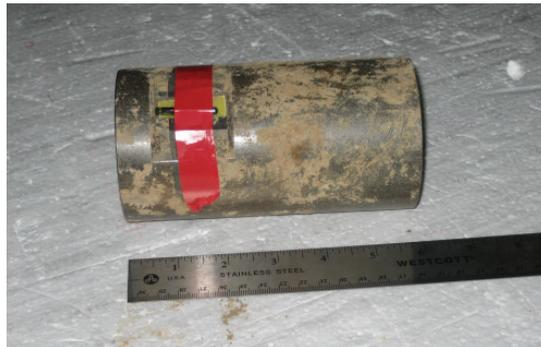
Fig. 15. Munition surrogate later buried at Aberdeen Test Center. The tag is evident below the red tape.
